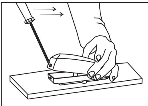
Insert a small 1-1.5mm flat screw driver into the slot at the back of the housing and lever the lid open.
